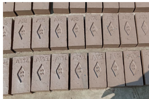
Fig. 4. Plastic bricks before burning
