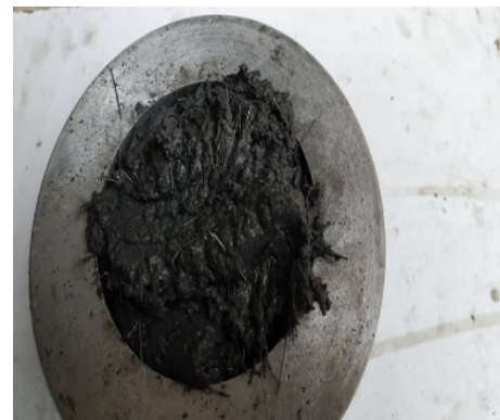
Fig. 2. Mini slump cone test for fresh concrete in the first phase of the trials
