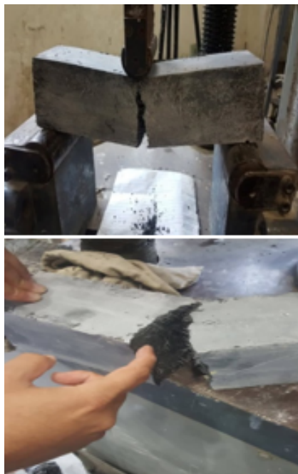
Fig. 14. Performance of the flexural strength tests on concrete cubes
