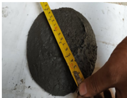
Fig. 10. Mini slump cone test for fresh concrete in 2nd phase of trials
