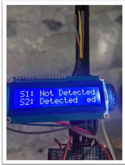
Fig. 5 Sensor 2 detects any motion, then displays "Detected," and the LED light goes on
