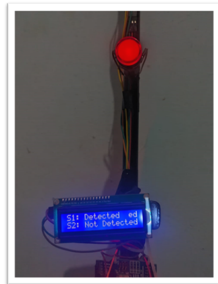
Fig. 4 Sensor 1 detects motion, then displays "Detected," and the LED turns on
