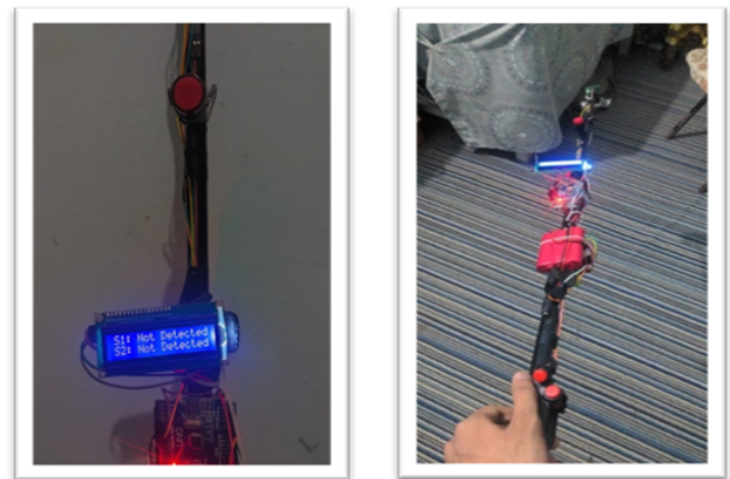
Fig. 3 The system is powered on, and nothing is detected during searching; the display shows "Not Detected," and the LED light is off.
