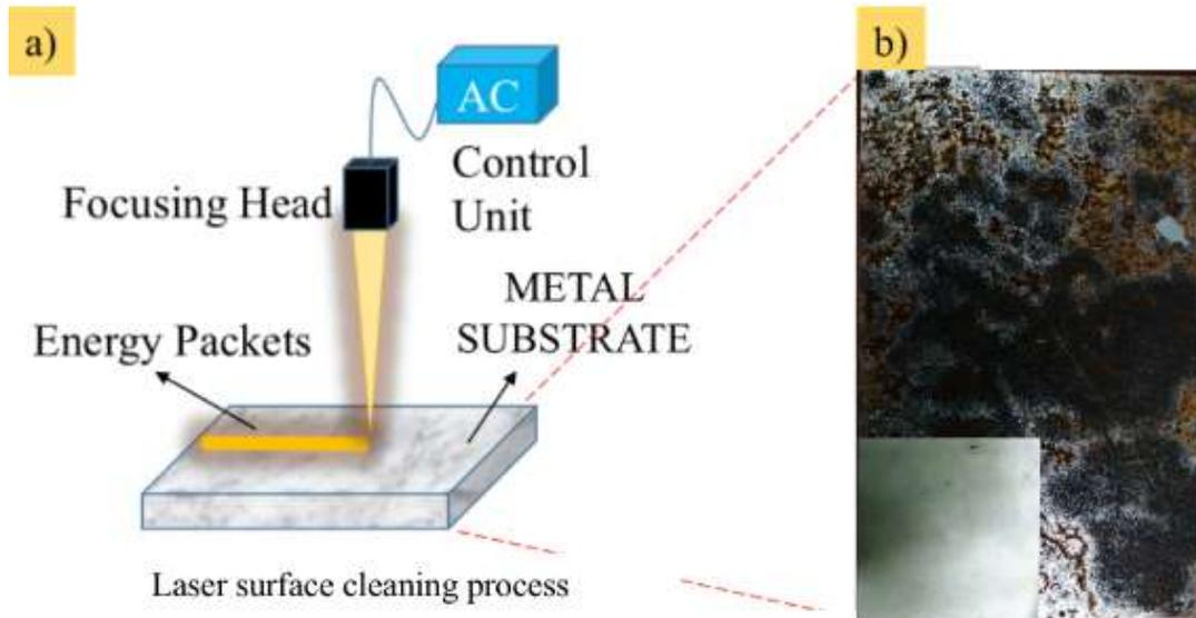
Fig. 2. a) The schematics for laser colour marking and (b) laser corrosion removal sample
