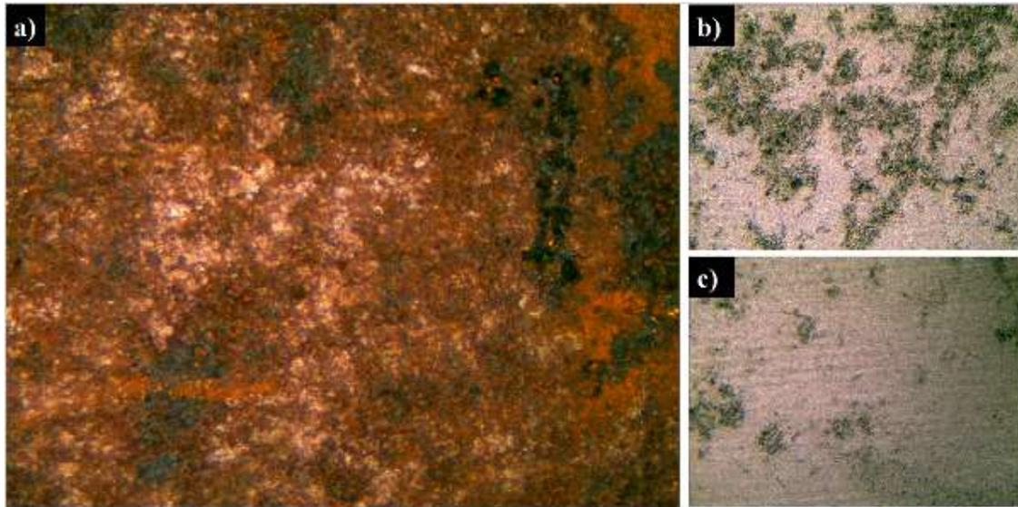
Fig. 4. Optical image of a) corroded SS304, b) LCR with retained black stains and (c) cleaner portion of LCR process
