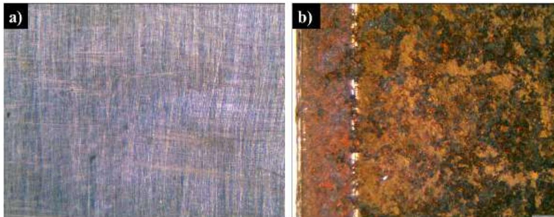
Fig. 3. Optical image of (a) as received samples and (b) corroded SS304
