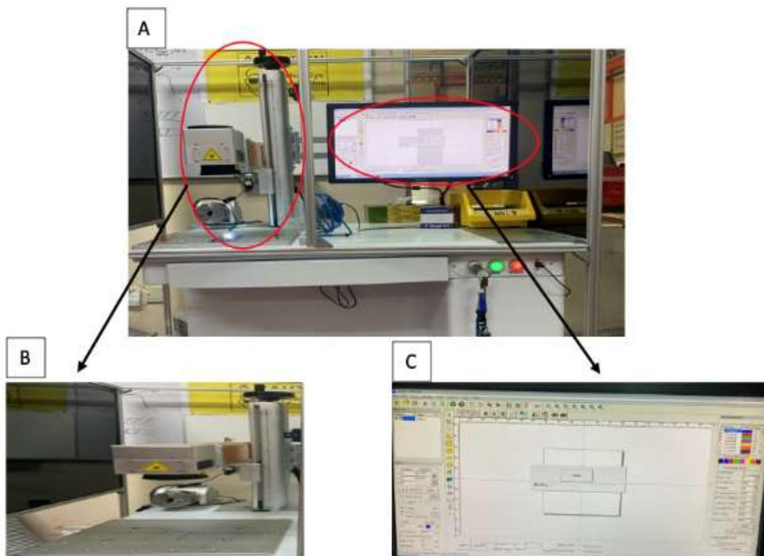
Fig. 1. a) Fiber laser machine b) Laser source with focus plane and c) software for laser cleaning machine (EZCAD)
