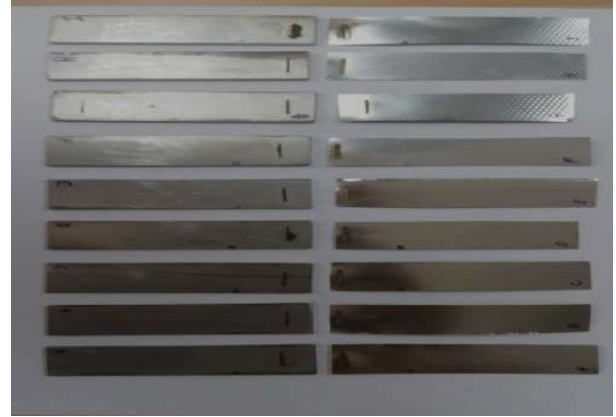
Fig. 3. Welded specimen arranged in alphabetical order from bottom to top after tensile testing
