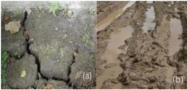
Fig. 2. (a) Shrinkage and (b) swelling of expansive soil
