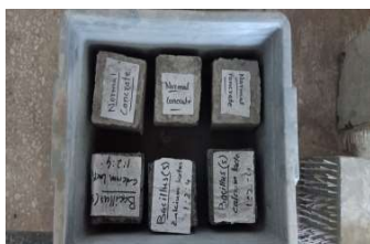
Fig. 5. Curing of concrete specimens
