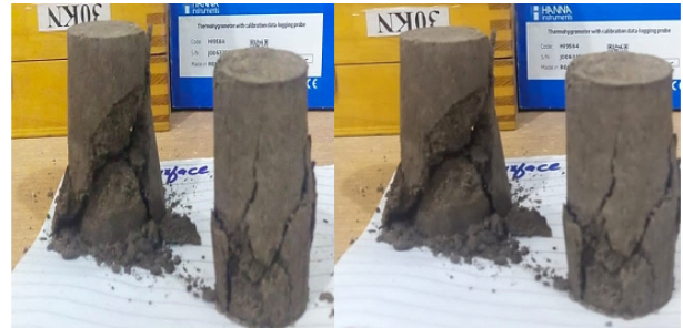
Fig. 16. Failure pattern of soil sample 1 (surface and 1meter deep) of the unconfined compression test (UCS)
