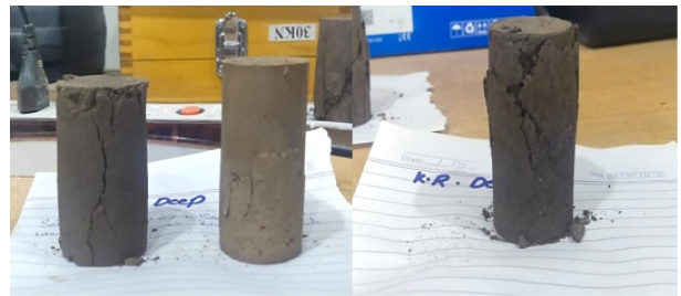
Fig. 17. Failure pattern of soil sample 2 (surface and 1meter deep) of the unconfined compression test (UCS)
