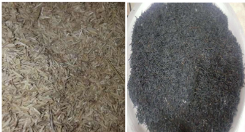
Fig. 2. RHA Before and After Burning
