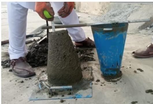
Fig. 6. Slump cone test of concrete
