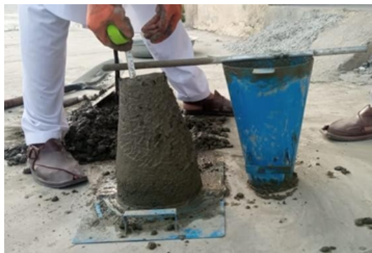
Fig. 6. Slump cone test of concrete
