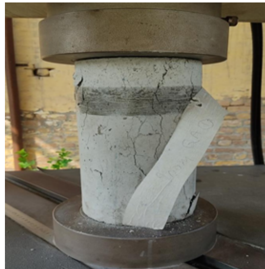
Fig. 8. Concrete sample for testing
